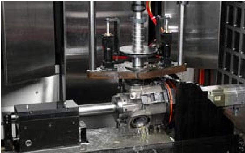
Ball screws achieve multiple Gs of acceleration with very high linear cycle speeds to meet the rapid reversal move profiles in the new Sunnen design.
