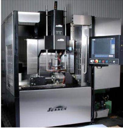
The SV Series, including the SV-200 and SV-1000, features the new tool stroking system with ball screw motion control to produce a true vertical stroke, resulting in greater control and higher accuracy in bore size and finish.
