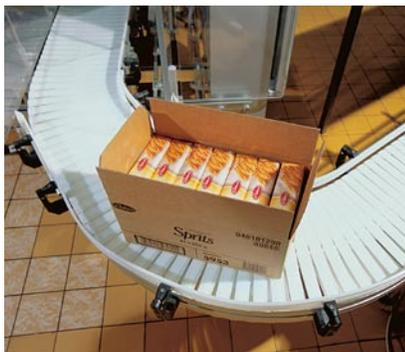
Boxes with individual packages of cookies are conveyed on a 12 in. chain that is also part of the VarioFlow program. Implementation of such a radius directly after a packaging machine is possible without a curve wheel thanks to an integrated bearing.
