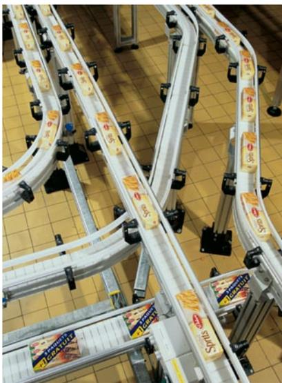
In some section, the conveyor section looks a bit like a roller coaster. United Biscuits uses various widths depending on the package. The 3 in. chain for individual packages and 6 in. for triple packs are able to run so close next to and below each other because of an integrated bearing in the VarioFlow.
