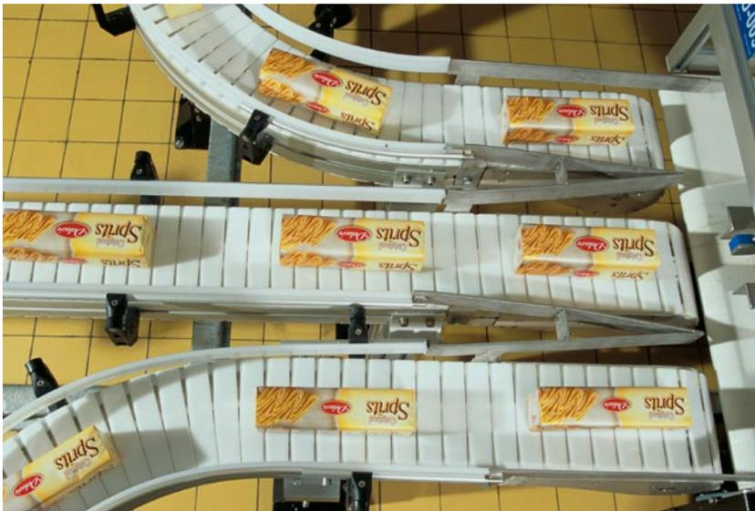
The VarioFlow chain conveyor from Rexroth does not need any cure wheels, since the bearing is integrated in the curve.
