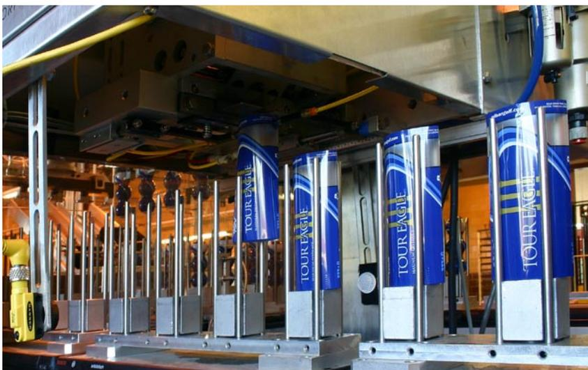
Four plastic sleeves are automatically inserted into the four nests of the fixture, mounted on Bosch Rexroth TSplus conveyors
