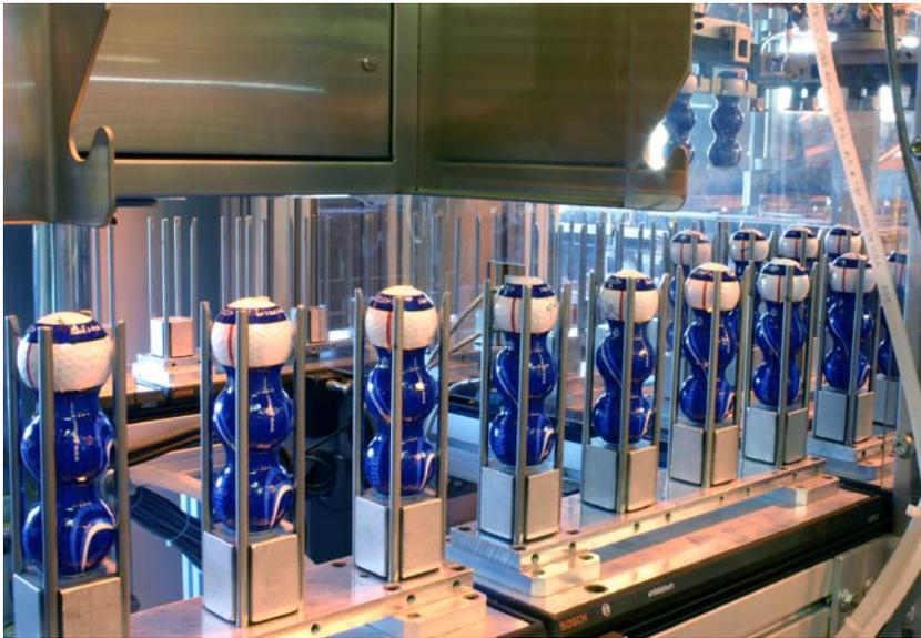
Sleeved Wilson golf balls after heat-shrinking carried on Bosch Rexroth TSplus conveyors
