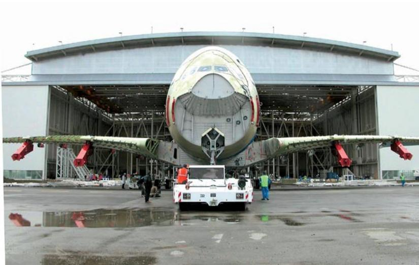
Whether in the hangar or at take-off position: The TPX 500 S towbarless aircraft tractor shoulders the mightiest aircraft in the world, the A380 Airbus.
