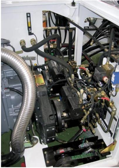
Both A4VG pumps incorporating the proven DA control system supply the power for the TPX 500 S.
