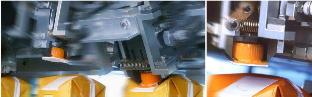
The spouts are attached to the closed cartons via an applicator. Exact positioning of the applicator is vital in this stage.
