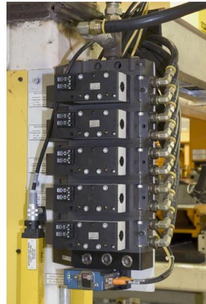
Pneumatic directional control valves plug into the EtherNet/IP-equipped Series 261 manifold. The valves use the Bosch Rexroth Drive & Diagnostic Link (DDL) to provide sophisticated diagnostic monitoring down to the solenoid level.
