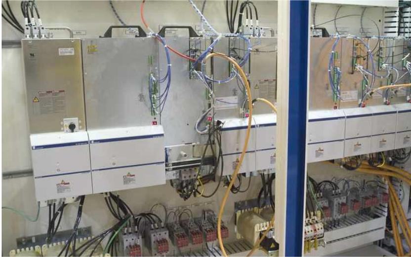
Bosch Rexroth DIAX04 servo drives control the horizontal movement of blanks.
