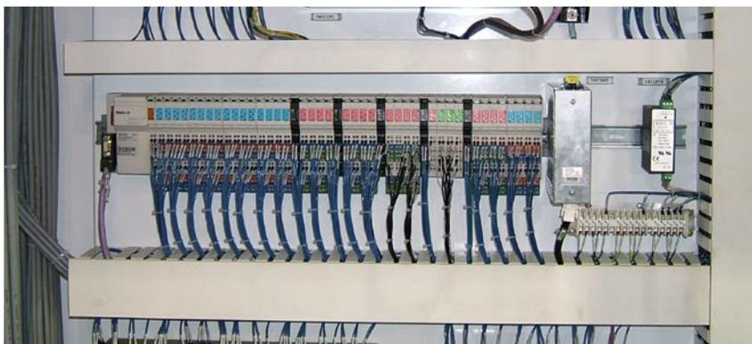
Ingersoll's machine takes advantage of distributed digital intelligent devices such as the IAC-R hydraulic valves, Fieldbus I/O, and electrical drives from Rexroth to significantly shrink panel space and wiring requirements.
