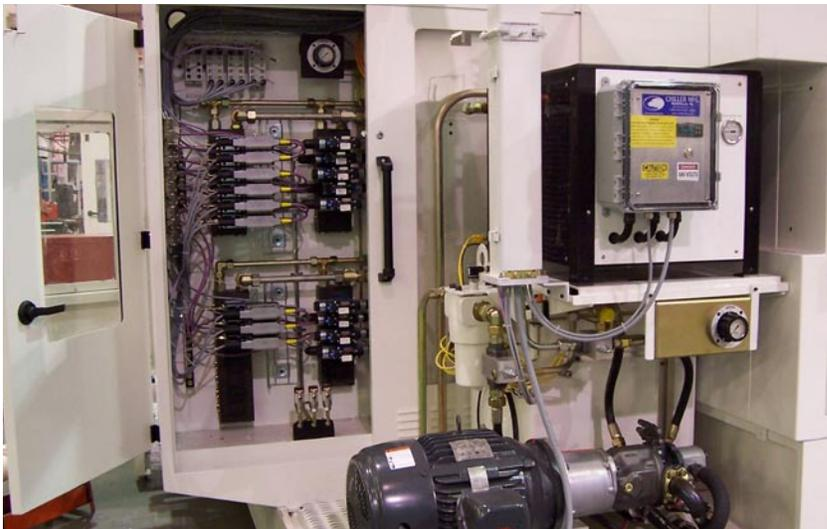
Using Rexroth IAC-R integrated axis controller proportional valves, Ingersoll CM Systems made its machine 25 percent more compact.
