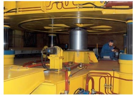
This is how the platform of the caterpillar transporter is raised, lowered and rotated.
