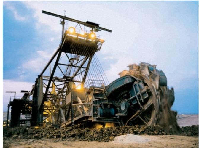
(Left) Extraction area worked by the Lignite Corporation in Neyvel in India. (Right) Huge bucket wheel excavators like these produce a tremendous quantity of excavated material, which is transported away on conveyor belts.
