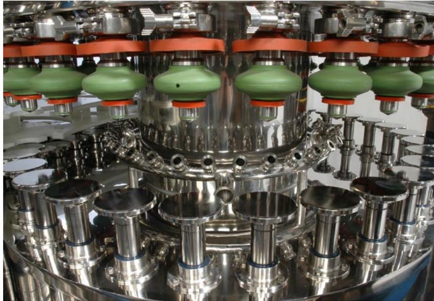
Using pneumatics for washdown applications in the beverage industry is an advantage because of low maintenance costs and reduced downtime.
