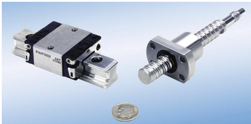
Rexroth engineers devised a custom electromechanical solution using their size 15 Ball Rail® driven by a precision Rexroth 12 mm ball screw in the T5 accuracy class to achieve the stiffness critical to smooth, vibration-free movement.
