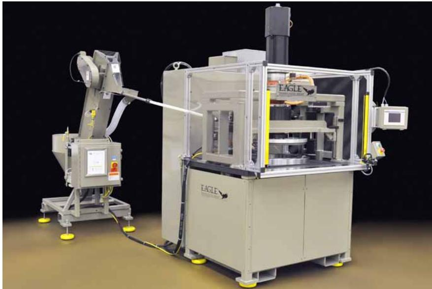
Eagle Technologies used a Rexroth drive and control platform to reduce components while improving output, durability and safety functionality on its power plastics welding machine.
