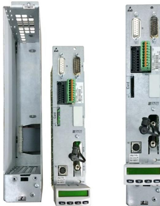
Located in the control cabinet with the drives, the HAC provides the physical framework (left) where an individual drive system control card, or section, could be inserted (right) to provide the analog conversion for the master encoder signal between the DiAx drives and the IndraMotion MLC.
