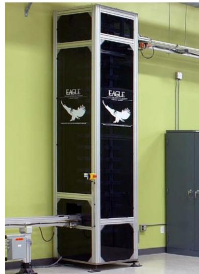
Using Rexroth aluminum structural framing, Eagle Technologies saved Ophthonix valuable floor space with this custom FIFO vertical buffer to transport trays to an overhead cooling line.
