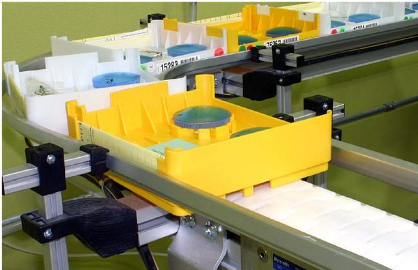
Rexroth uses patented curve technology to reduce friction in curves, allowing trays to accumulate in the curve while using fewer drives to save on system costs.
