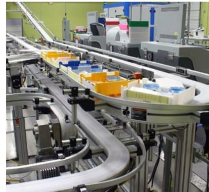
With the Rexroth conveyors, standard robotic processing trays can accumulate in curves as they are routed to various stages of production.
