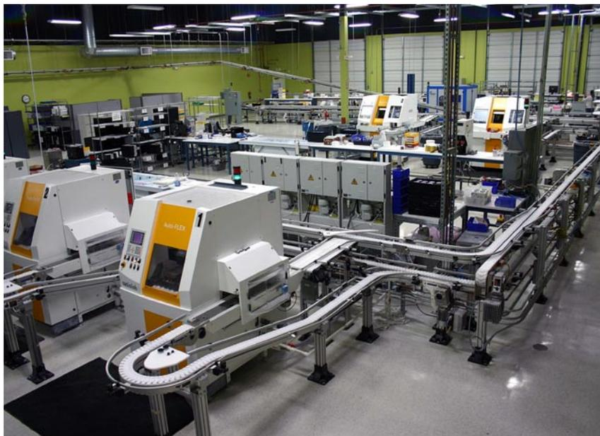
With over 1,000 feet of conveyors, lens polishing equipment can easily connect into the main line as future production needs increase.
