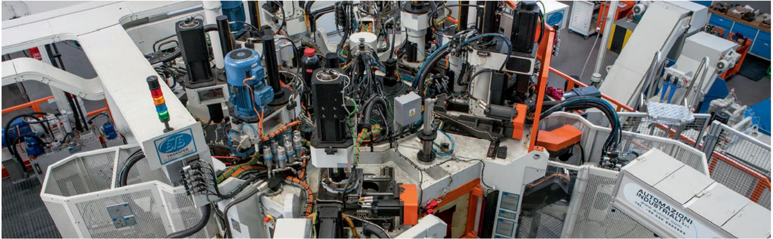
Seppelfricke Armaturen: Rotary transfer machines with Rexroth CNC control
