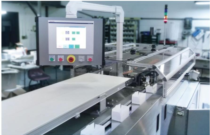
Veronica's automation control is from the IndraMotion XLC motion-logic automation controller, which supports up to 16 axes of motion and enables fast changeovers to different size cartons.
