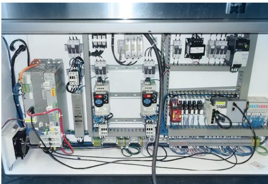
The compact size of the Veronica's control cabinet is enabled through the use of the IndraDrive Mi drive-integrated servomotor system, which removes the servo drives from the cabinets and incorporates them into the motor housing.
