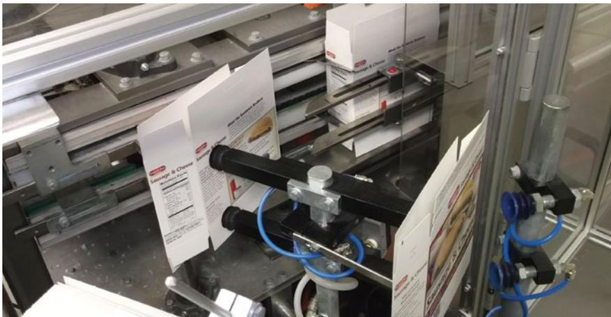
The Veronica is a fast and reliable machine for erecting cartons from flat paperboard blanks and precisely transporting and synchronizing the loading, closing and gluing of the cartons.
