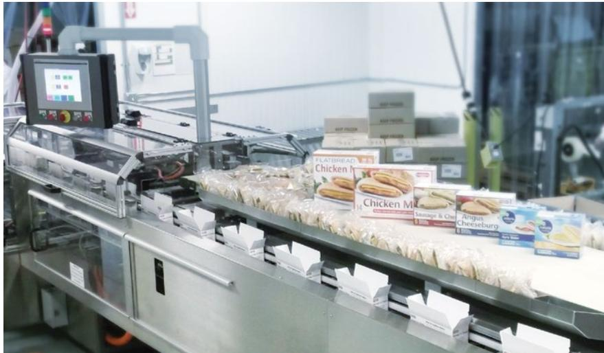
Ultra Packaging's Veronica vertical cartoner provides an efficient, compact cartoning solution that enabled Kangaroo Brands to automate erecting and processing the cartoning of its fast-growing line of pita pocket sandwiches.
