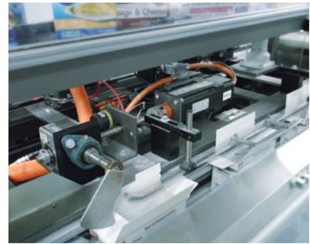
The IndraDrive Mi is engineered to fit into tight machine spaces and features a single cable combining power and communications. It is used to drive multiple axes on the Veronica, including automated closing and sealing of the carton flaps.
