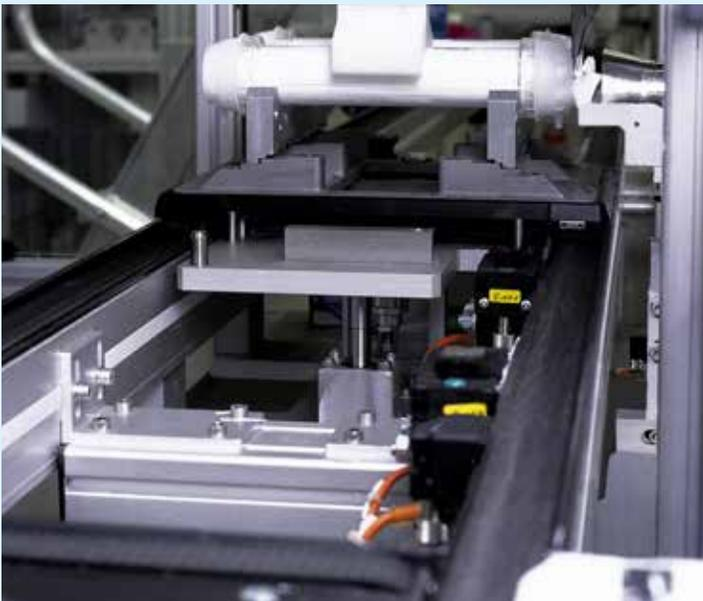
Belt media (flat or toothed) is ideal for transporting small parts and light payloads. Most belts feature an electrically conductive coating and are ESD-ready. Most belts are cleanroom-ready and are commonly used in “clean” applications, including medical device and electronics assembly.
