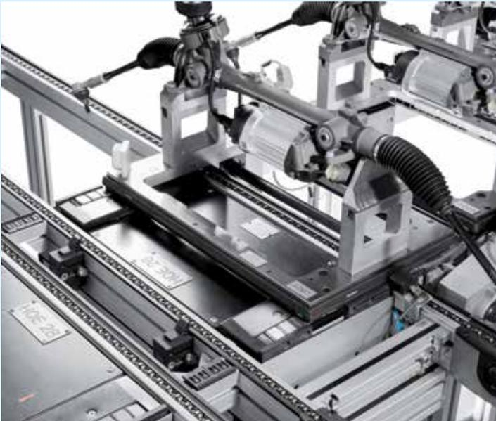
Roller chains are available in many designs (steel, plastic, accelerating) and can be used in the most challenging environments. The power-and-free design creates a low-friction surface, allowing roller chains to convey heavy payloads. Most roller chains are also bi-directional, making them suitable for reversing applications.
