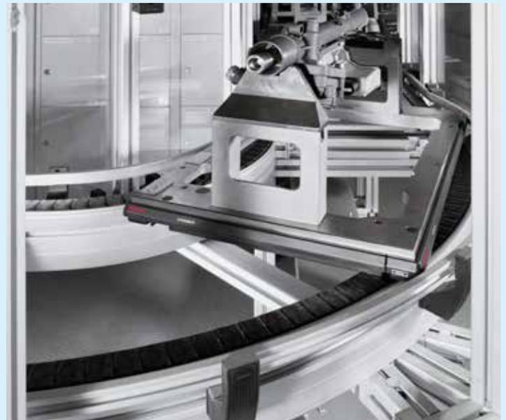
Flattop chains are capable of supporting heavier payloads, and their side-flexing design makes them ideal for use with curves and for maintaining leading-edge pallet orientation. Flattop chain caps commonly overlap each other, which makes this media very “fastener-friendly.”
