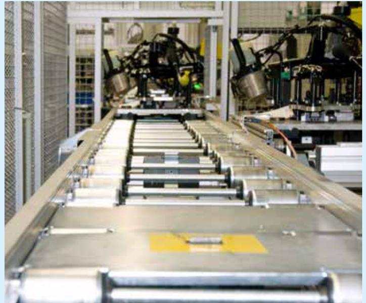
Powered roller conveyors generally have the highest payload capacities and offer the most robust conveyance solutions. They're also very quiet in operation and have low maintenance requirements.
