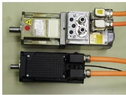
Some drive/motor models mount the electronics on the back end of the motor, which is an obvious disadvantage in component size compared to the IndraDrive Mi (bottom).
