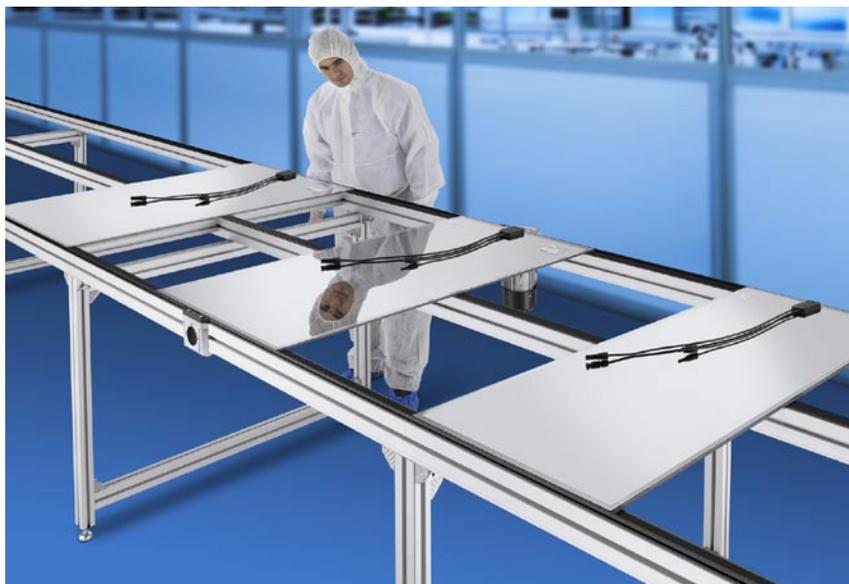
In the solar industry, production methods for processes such as stringing and lay up, vary greatly from one solar panel manufacturer to the next. As a result, solar industry requirements often generate a variety of custom conveying/material handling requirements.
