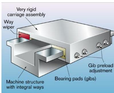
FIGURE-1: Traditional boxway slides require complex lubrication systems and gib adjustment.
