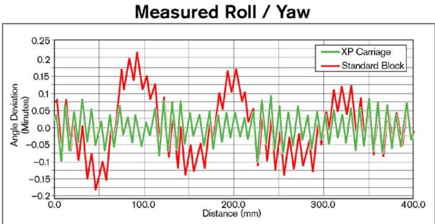
FIGURE-7: Enhancements to the ball raceways result in 60% less deviation as the high-precision runner block travels along the rail.
