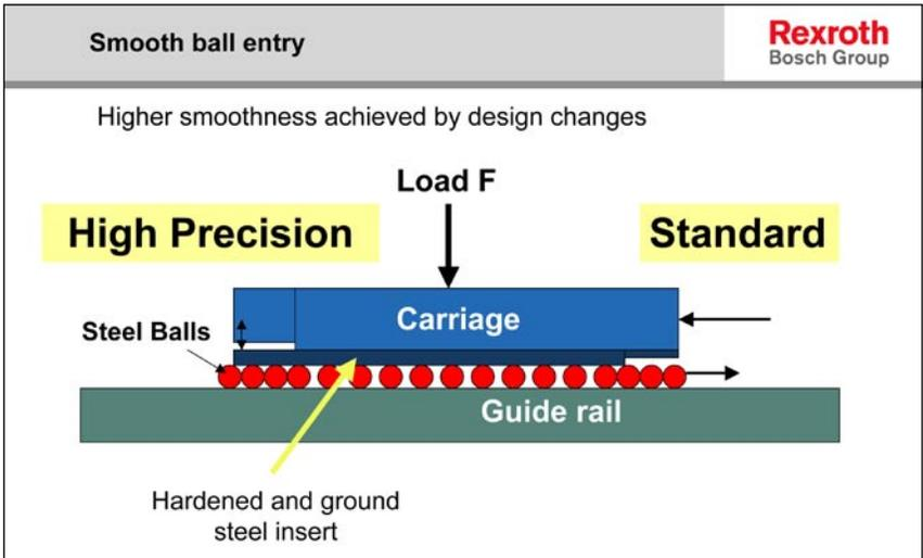
FIGURE-6: Split view shows how steel insert works with balls on the high-precision product (left) vs. standard product (right).
