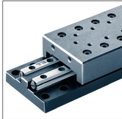
FIGURE-2: Cross roller slides are the most commonly used product for high accuracy applications but typically do not work well for strokes over 600 mm.
