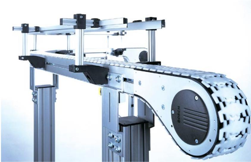
Changes on-the-fly: Adjustable guide rails provide flexibility to quickly adapt to a wide range of container shapes and sizes, reducing time-to-market cycles.
