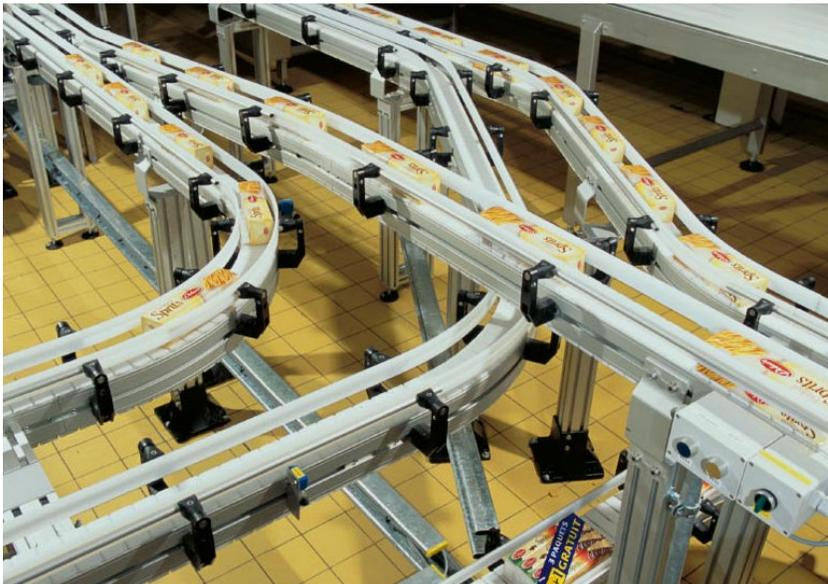
Modular conveyors form a “highway” system to coordinate product flow and balance production in high-speed packaging operations, and are the foundation of an adaptable packaging operations strategy.
