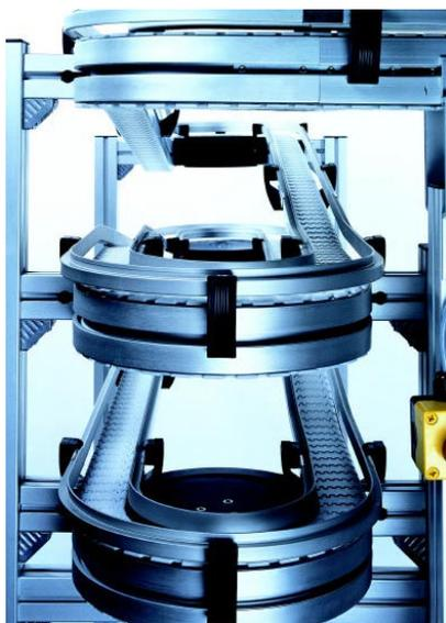
Maximum density, maximum efficiency: buffering conveyor systems—like this vertical inline spiral accumulation system—offer ultra-compact accumulation to minimize floor space and keep production going.
