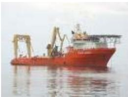
(Norman\_Installer.jpg) Norman Installer, equipped with 175 t MAHCS for installation of suction anchors at 2000 meter depth.
