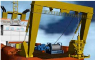
(AHC.jpg) Basic impression of a Rotating Active Heave Compensator ready to lower a subsea template.
