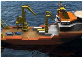
(AHC\_on\_deck.jpg) Top view of a Rotating Active Heave Compensator (in left corner) illustrating the compact construction, requiring far less space on deck.
