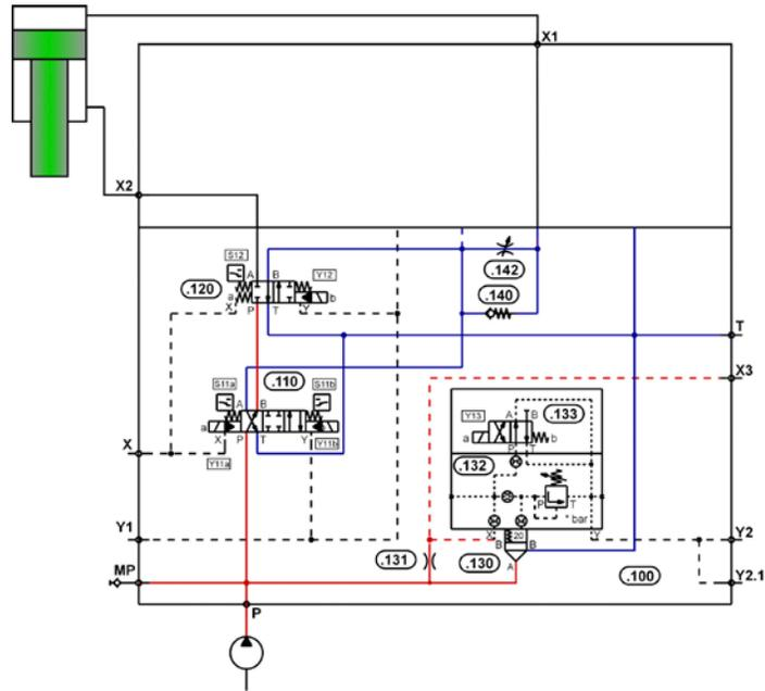
**Picture 3:** Valve #110 is stuck in the crossed position
