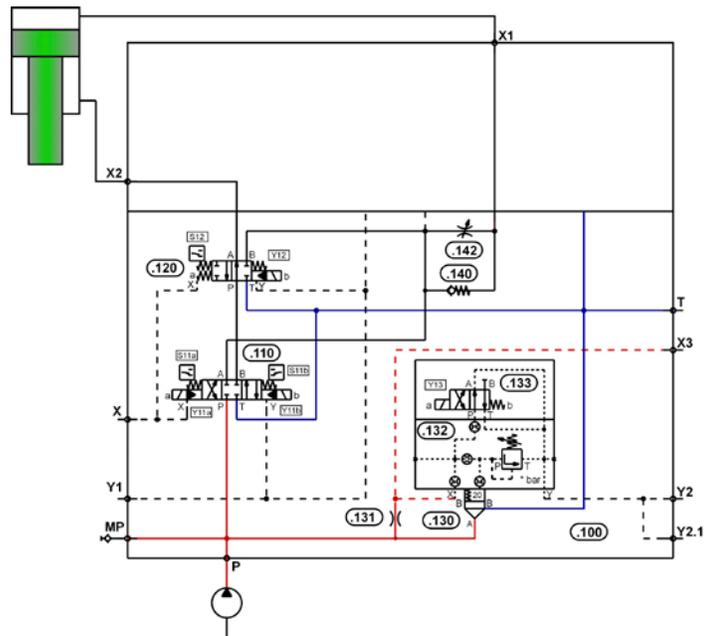
**Picture 5:** Valve #120 is stuck in the activated position
