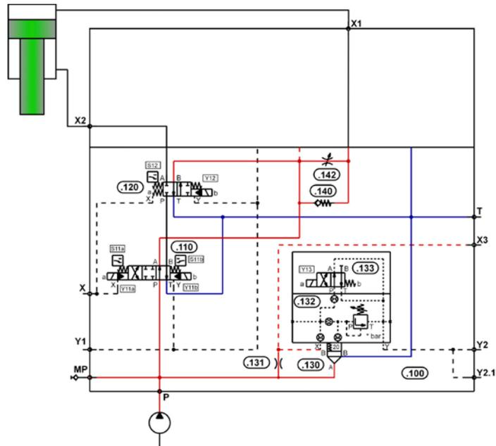
**Picture 4:** Valve #110 is stuck in the parallel position
