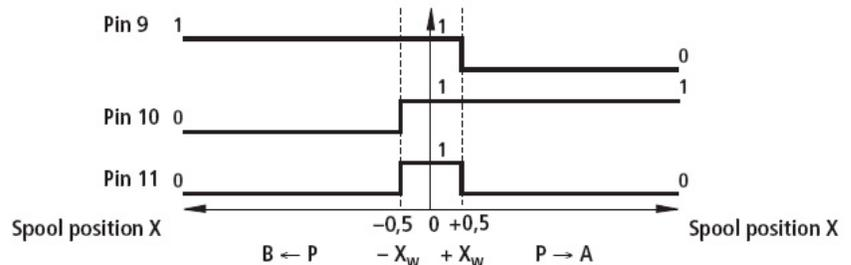
Picture 11: Switching logic of spool monitoring in proportional valve
