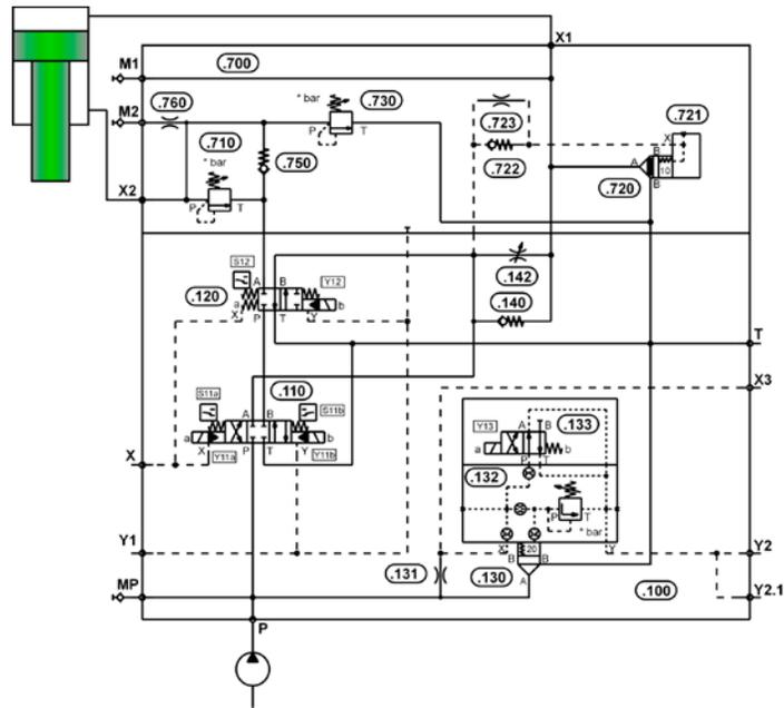
**Picture 2:** Hydraulic Press Control with Safety Circuit
