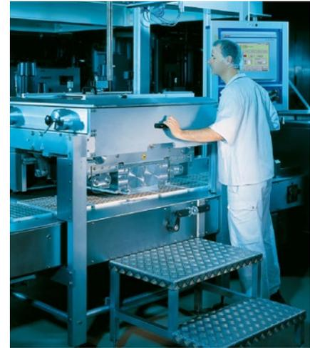
By using a standard (non-safety) input with no redundancy or diagnostics, it is possible that a single failure could cause loss of the stopping function and allow rapid motion toward the operator's hands.
