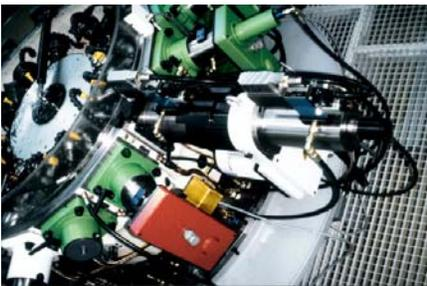
Hydraulic linear drive with revolving transfer machine.
