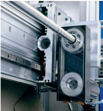
Electromechanical feed drive with static screw spindle and nut driven via synchronous belt.
