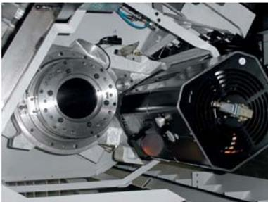
Main spindle drive with housed motor.
