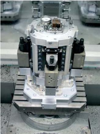
Hydraulic clamping fixture for valve housing.
