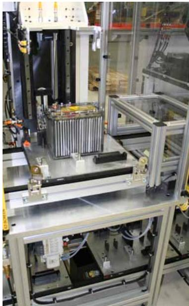
Rexroth TS pallet-based systems offer a wide range of options for routing, handling and positioning heavy battery components.
