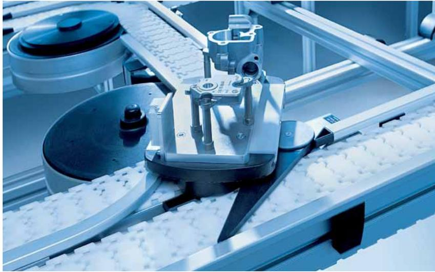
Systems like VarioFlow are typically used for lighter-duty processes in battery assembly applications (e.g., individual lithium-ion cell components a few inches square) but they are capable of handling considerable weight and size, and offer high chain tensile strength (up to 1,250 N).
