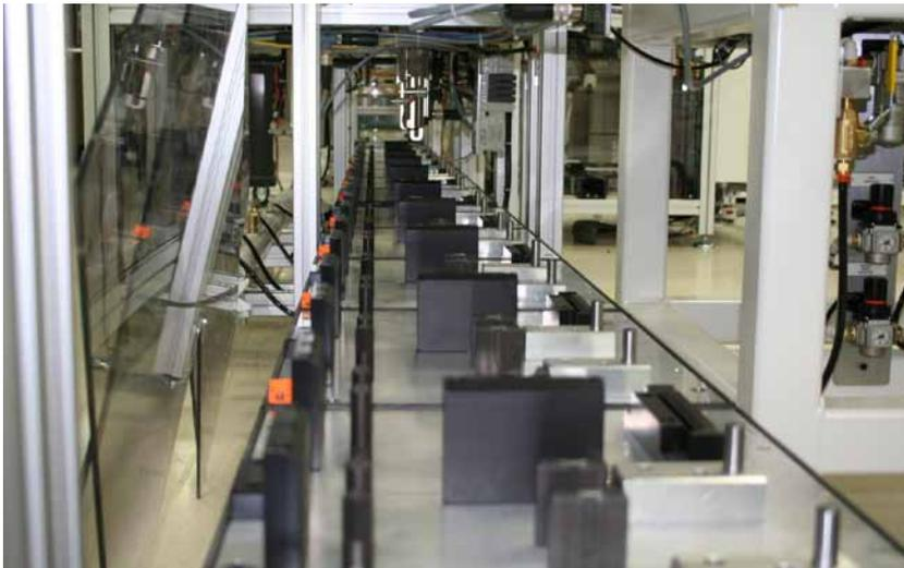
Modular conveyor components, such as Rexroth's TSplus conveyors, are at the heart of many battery assembly systems, increasing line productivity while reducing the potential for damage to the product.
