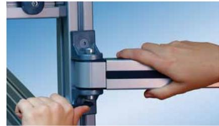
If lab equipment frequently needs to be repositioned or reconfigured, look for T-slotted extruded aluminum structures with simple bolt-together designs that allow for speedy reconfiguration of individual processes or even entire labs.
