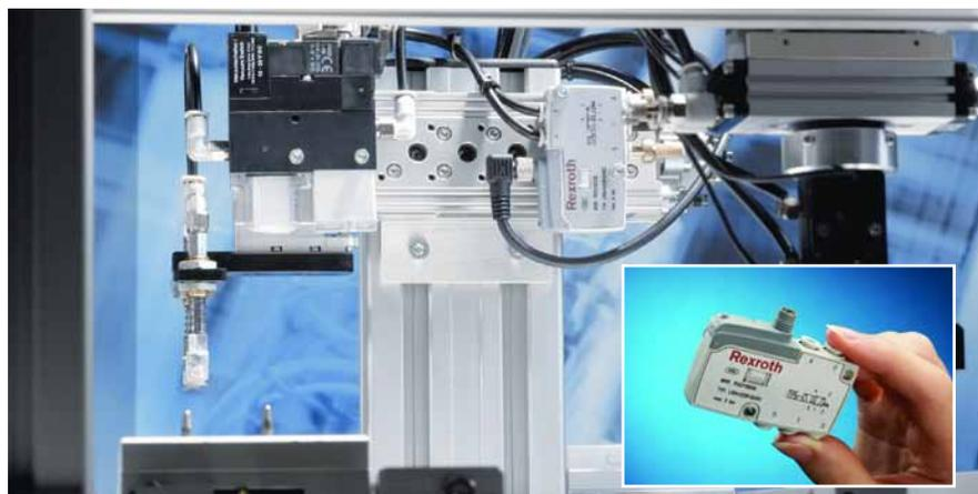
Since air losses can occur at distances as short as three feet, mounting pneumatic valves close to the actuators they control will reduce the energy needed to deliver the air. Pneumatic component manufacturers now offer smaller, lighter chemical-resistant valves that can be mounted directly on the machine instead of in a control cabinet, resulting in significant energy savings.
