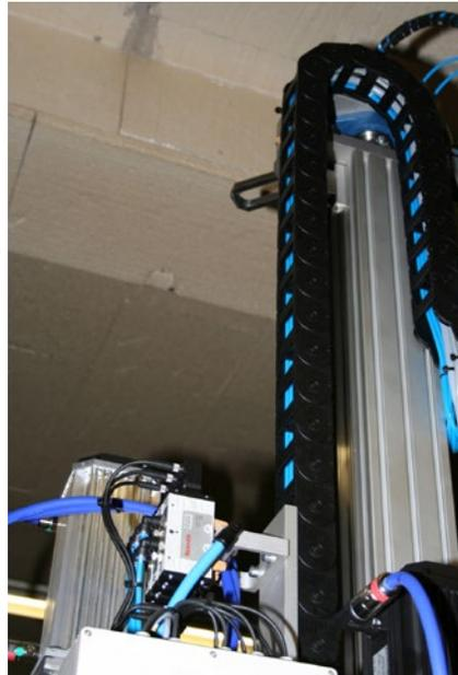
Clean and careful cable management is often overlooked, but can help you make sure that even tight spaces don't cause problems. Failure to consider cable management can result in shortened system life, physical incompatibility with the ultimate operating environment, or even fires.
