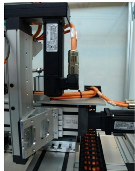
Getting the right motor is critical, which means matching it up to the overall system's mechanical components. In other words, electrical system design can only occur once the mechanical design has been fine-tuned to match the performance specs of the application.
