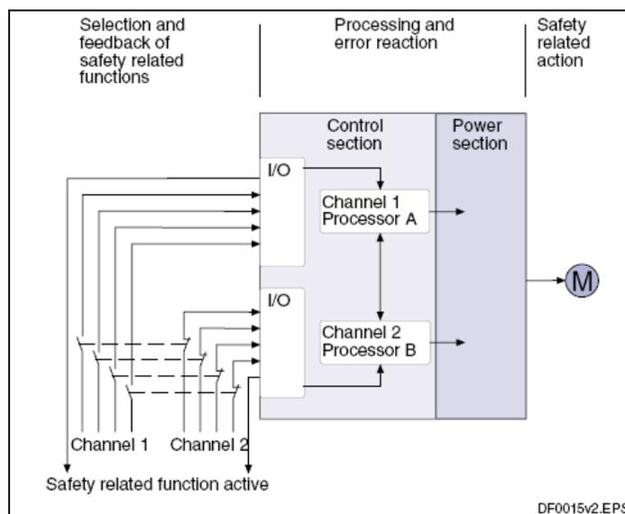
Two-channel safety processing cross-compares parameters to catch errors and activate safe standstills.
