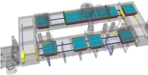
(Figure 1) Vacuum carrier system with 18 stations. The products move from Load lock IN position through the process area, to the Load lock OUT station.
