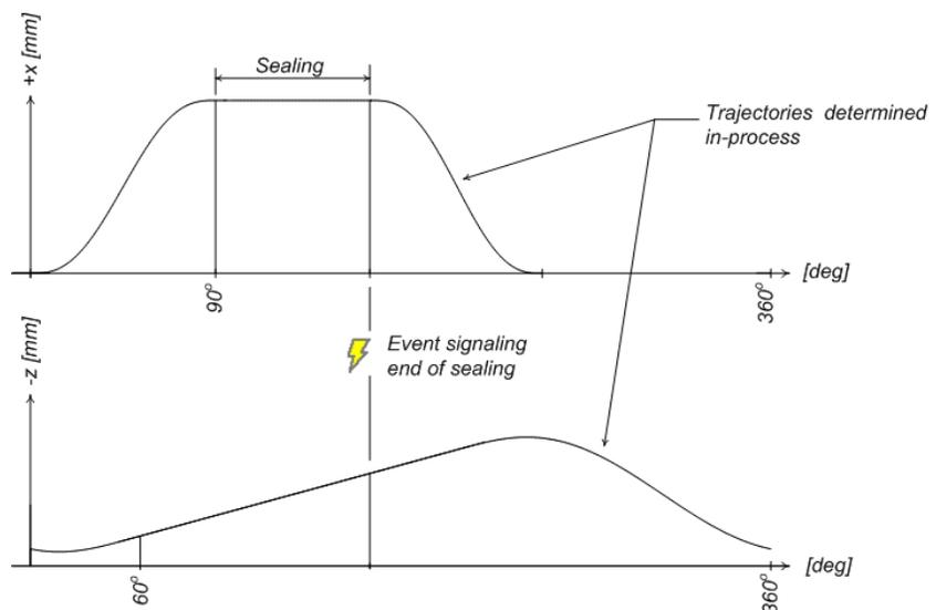
**Figure 3.** In the event-driven motion model, the sealing bars open as soon as the event occurs and (after some overlap) the bars return to their start position. Note that in this scheme the return trajectory is not predetermined as the event may occur at any time.
