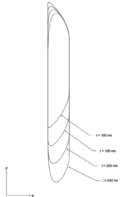
**Figure 8.** Sample of trajectories generated by Flex Profile as a function of the sealing time  $t$ . Note that the trajectory is calculated in-process and that the event which signals the end of sealing may occur at any time during the sealing process.
