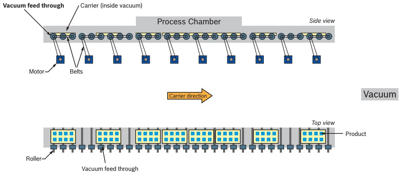
**Figure 2:** Roller transport system
