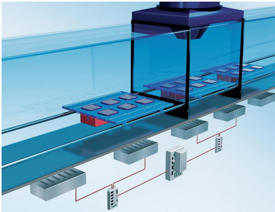
**Figure 1:** Inverted linear motor deposition chamber example
