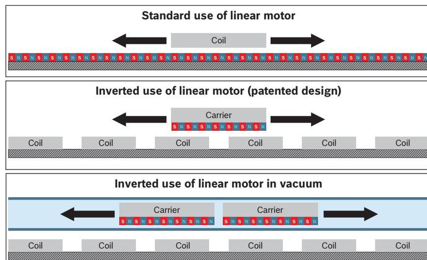
**Figure 3:** Standard and inverse linear motor systems
