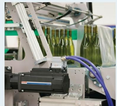
Integrated motor/drive systems are especially suited for modular machines, such as packaging equipment, where line extensions are added for different products.
