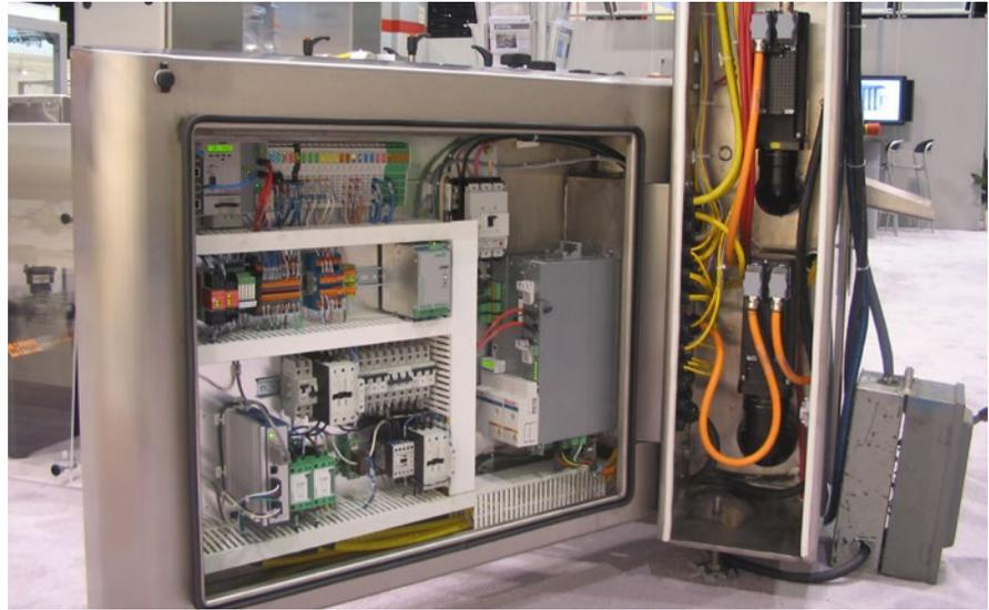
With integrated servo drive/motor technology, the drive electronics are relocated from the control cabinet and mounted directly on the motor at the machine.
