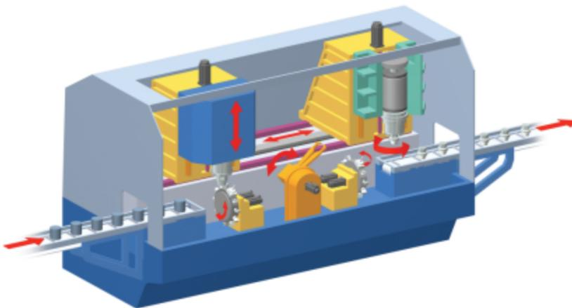
**Figure 8:** Distributed intelligence in the automotive industry. Distributed intelligence is used on machining transfer lines. Transfer lines are constructed of several machining stations performing different or similar machining tasks such as drilling, tapping, and milling.
