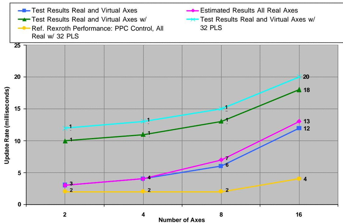
**Figure 2:** This chart shows the baseline, Rexroth controller, compared with a competitive PLC-based controller. Notice how the Rexroth controller (gold line) stays flat regardless of the number of axes, finally rising after eight axes. In contrast, the competitive controller's processing speed varies greatly depending on the number of axes, whether these axes are real or virtual (real axes normally take more processor cycles), and the number of Programmable Limit Switches (PLS) required.
