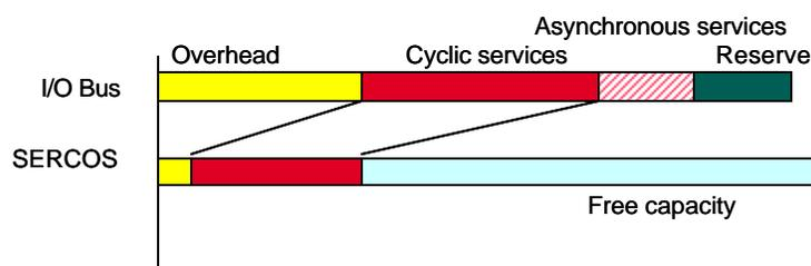
**Figure 4:** SERCOS interface is deterministic for motion control compared to an IO fieldbus communication.
