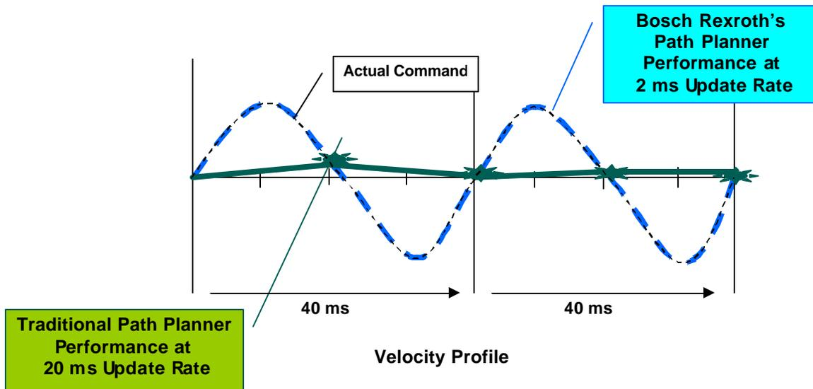
**Figure 3:** This figure shows practical implications of this lack of processing speed. The dotted line is the velocity command path generated by the control program. The blue line is a velocity path generated at a 2ms update rate, while the green line is a velocity path generated by a competitive, PLC based system running at a 20ms update rate. It is apparent which system will follow the calculated path more accurately.
