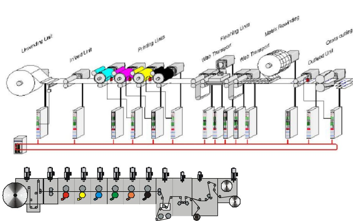
**Figure 7:** Distributed intelligence in printing and converting. Newspaper printing presses, unwinders/rewinders, coaters and laminators are some of the applications taking advantage of distributed intelligence. Other applications include register control, tension control, winder and dancer control, electronic cams, and electronic gears.
