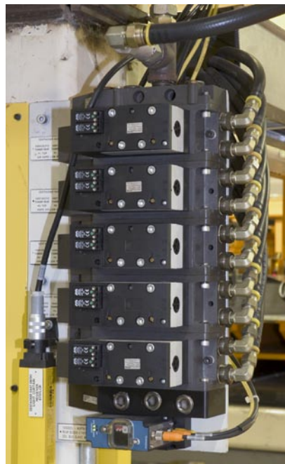
This Rexroth Series 261 pneumatic manifold is EtherNet/IP-equipped, making it easier to integrate into an application.
