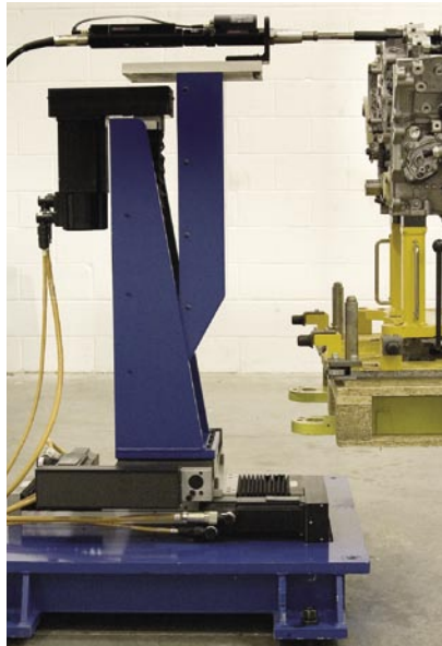
The PLP is a servo-driven, three-axis Cartesian robot that serves as an economical alternative to traditional custom pallets.
