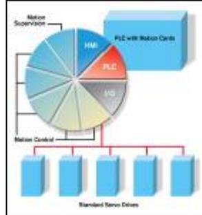
Machines are becoming more motion-centric; as axes increase, machines can become more flexible and productive. Distributed intelligence is designed around the motion-centric machine, so you can add more intelligent digital drive axes without having to upgrade or change the control platform.
