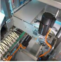
**ADV2578\_01.jpg** The intelligent drive monitors itself as well as the feedback from the motor it drives – including torque, speed, acceleration and other parameters.
