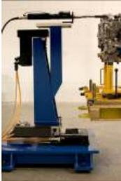
*(Programmable Lift Platform)* The concept of the Programmable Lift Platform (PLP) replaces expensive pallets and robots with easy-to-build programmable gantry style platforms that use modular automation components such as ball screws, linear elements, PC control and electric servo motors and drives.
