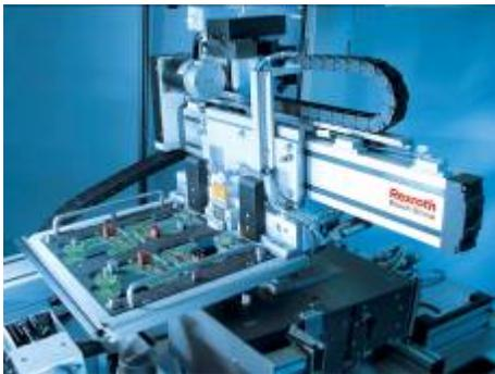
(BRL\_CKK\_App.jpg) Cartesian robots are ideal for precise operations like electronics assembly.
