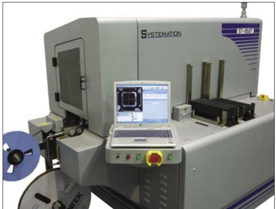
The Systemation ST 868 is a High Speed Semiconductor Inspection and Packaging system capable of processing up to 15,000 chips per hour (four per second).
