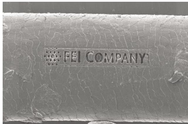
Extremes in motion control performance—extreme throughput, extreme stability—are represented by this image of the FEI Company's logo carved into a human hair (diameter  $\approx$  50  $\mu$ m) with an ion beam and captured by FEI's Nova NanoLab 600 scanning electron microscope.
